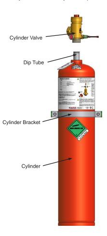
**Cylinder Valve**: The automatic release of FM-200® is controlled by a forged brass, differential pressure operated cylinder valve connected to the neck of the cylinder. The valve assembly is shipped with an antirecoil safety plug installed in the discharge outlet and chained to the cylinder valve.
