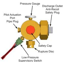
The cylinder valve has four key features:
