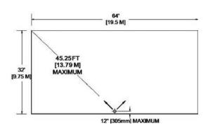
180° Sidewall Nozzle (2 Port) Arrangement
